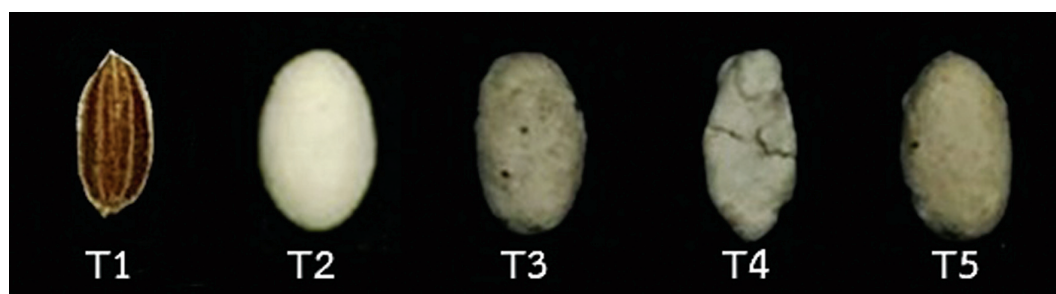
Figure 1 Physical characteristics of lettuce seeds pelleted with different filler materials. T1 = Control, T2 = pelleted seed + calcium sulfate, T3 = pelleted seed + zeolite, T4 = pelleted seed + bentonite and T5 = pelleted seed + pumice.
